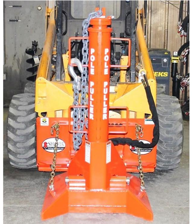
1. Position the skid steer behind the Utility Pole Puller.
