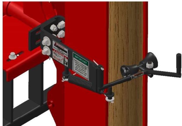
Drive Ram and Safety Arm with fence post.
