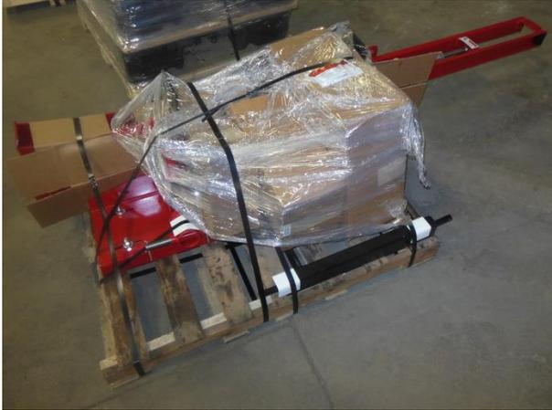
The Post Driver is shipped in several sections: The Driving Ram Assembly, Base Plate Assembly, Hose and Valve Carton, Safety Arm Carton, and with the Hydraulic Post Driver (HD-8-H-S, HD-10-H-S, & HD-12-H-S) the Tilt Cylinder Carton.
