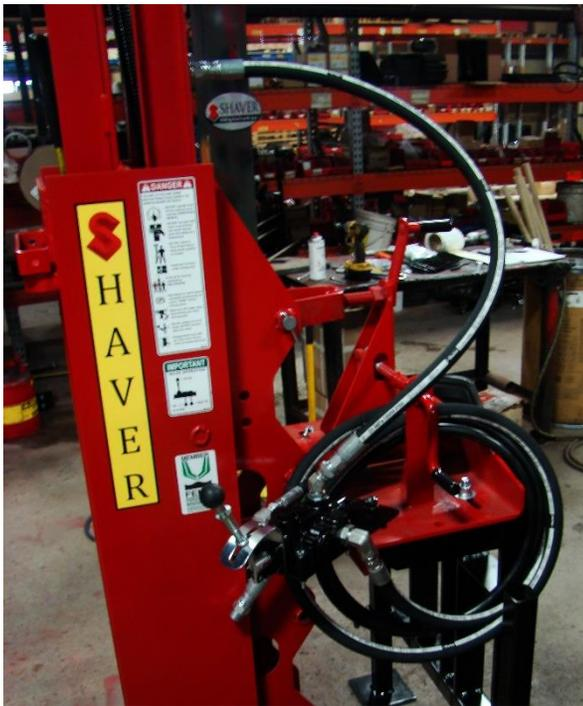
directly to the hydraulic reservoir of the tractor or skid loader.
