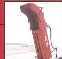
Telescopic chute extends by 28 inches (711 mm)
