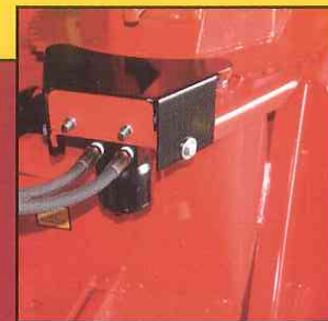
Orbital rotation mechanism with hydraulic motor at 300°.
