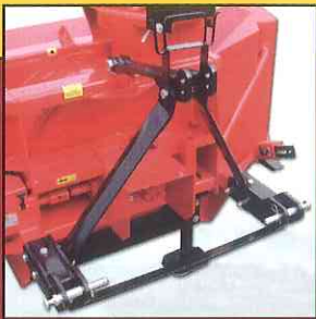
Heavy duty 3 point hitch adjustable in 2 positions.
