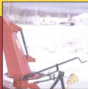
Manual rotation mechanism at 300° only for group I models.
