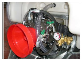
The pump can be identified from the data plate applied on it; the main data of pressure and flow are easy to find. Normally the pump must not exceed 550 rpm; a number of major tours does not improve performance but compromise the life and safety of the equipment. On the pump there is a safety valve calibrated to prevent the over pressure. Do not tamper with this valve for any reason and do not block the hose connected to it.
