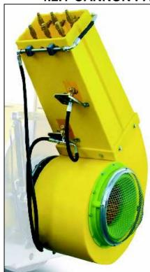
The cannon fan group has similar gear box like normal axial fan groups and the characteristics are similar too. The impeller has a centrifugal fan type capable to producing an air flow at high speed, guaranteeing a high spraying.
