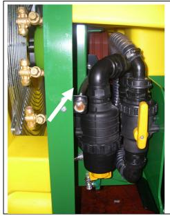
at the rear right side of the fan unit is installed a light indicating the oil level. If the oil level is not visible please top up by inserting the top of the fan where there is a priming plug.
