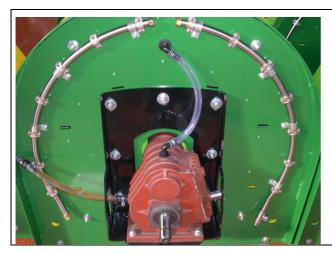
The gear box is made by a gear body with a gearing inside that increases the input power from the pump (supplied from the output joining shaft or keyed depending on the models) transmitting it to the impeller and consequently the operation using the output shaft.
