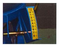
Important: Lever position expected for DTS/DTE is an approximate value, sulfur rate have to be checked doing a test outside plantation, not a proper dosage can cause important damage to crops.
