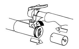
Remove the protective cover from the atomiser by pressing down on the tab as shown. Check by hand that the atomiser disc spins freely.
