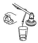
If the flow rate is not in the recommended flow rate range of 2 to 6 oz/min change the feed nozzle and repeat the above procedure. N.B. It is preferable to walk more slowly to achieve the required spray volume than to use higher flow rates.
