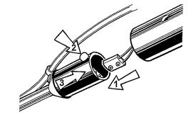
Screw the union nut (4) into the flow control valve.
