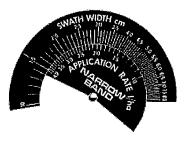
3. On the calculator disc align the swath (band) width (in cm) with the total volume application rate (e.g. 20 l/ha) as determined in 1, above.
