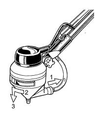
When refitting the atomiser disc it is important to ensure that it is correctly located in the atomiser cone housing and motor housing to avoid damage.
