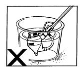
From time to time it may be necessary to clean the atomiser disc. To access the atomiser disc, the atomiser cone housing must first be removed.
