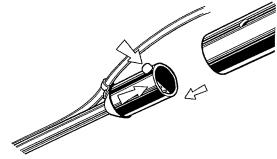
Connect the spray feed tube from the spray lance into the dual control switch on the handle.
