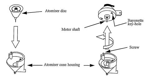
First, lower the atomiser disc into the atomiser cone housing ensuring that the disc shaft seats on the ball in the bottom of the atomiser cone assembly.
