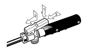
If the master electric switch is in the off position the dual control switch will regulate liquid flow only.
