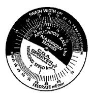
4. Having fixed the swath (band) width and application rate select the preferred walking speed (2km/hr = Slow, 3km/hr = Medium, 4 km/hr = Fast).
