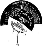
5. Read off the feed rate required to give the correct application rate. (e.g. 30 ml/min with 30 cm swath (band) width and walking speed of 3 km/hr to apply at a volume of 20 l/ha).
