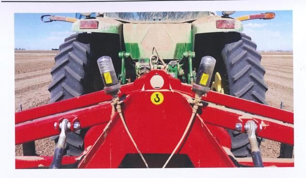
When you have finished to work or during the day check always to have enough grease for the next day. Otherwise go to the greasing position with a <u>manual</u> pump and fill the proper tank.
