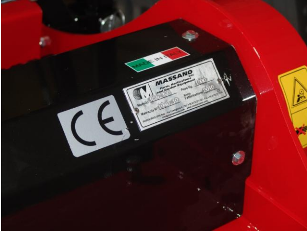
Location of the EEC plate on the machine
