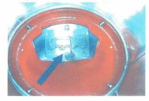
The base plate is shipped from the factory on the letter F, (top arrow in photo on left). This is the correct position for a centered spread with this style blocking plate.
