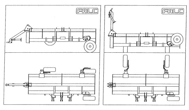
There is an easy assemble and use transport trolley available for the transport of the machine using the drive hook of the tractor. The more recently produced shredders are equipped with a series of holes to bolt the base of the rudder and the wheels. The transport trolley may be requested at the moment of purchase or can be applied directly by the user. In this case the user must check to ensure that the machine in his possession is adequately equipped.
