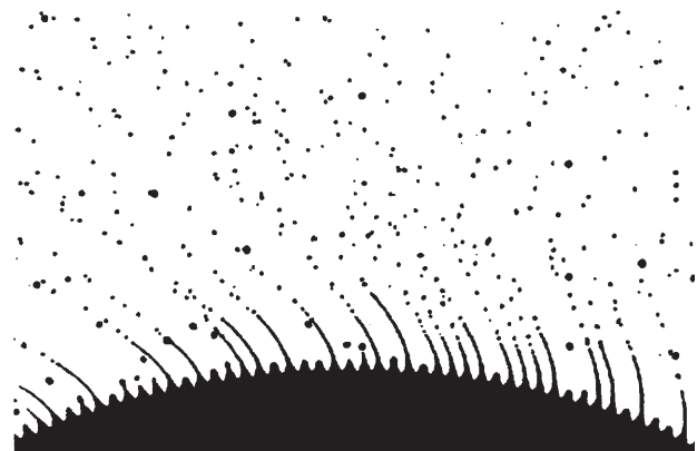
Figure 2. Single and Ligamental Droplet Atomisation.
