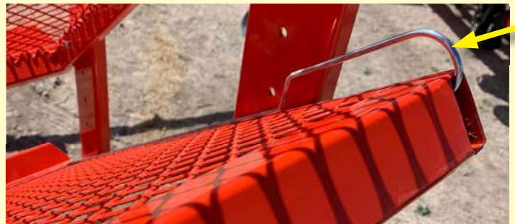
Clean-out rod to clean out soil/debris from throat and shoes.
